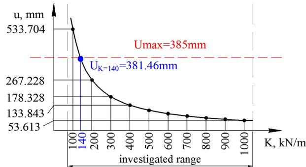
Fig. 4. The relationship between the stiffness of a damping bearing ( $K$ ) and the horizontal displacement of the bottom point of the building ( $u$ ) in the range from  $K=100$ kN/m to  $K=1000$  kN/m
